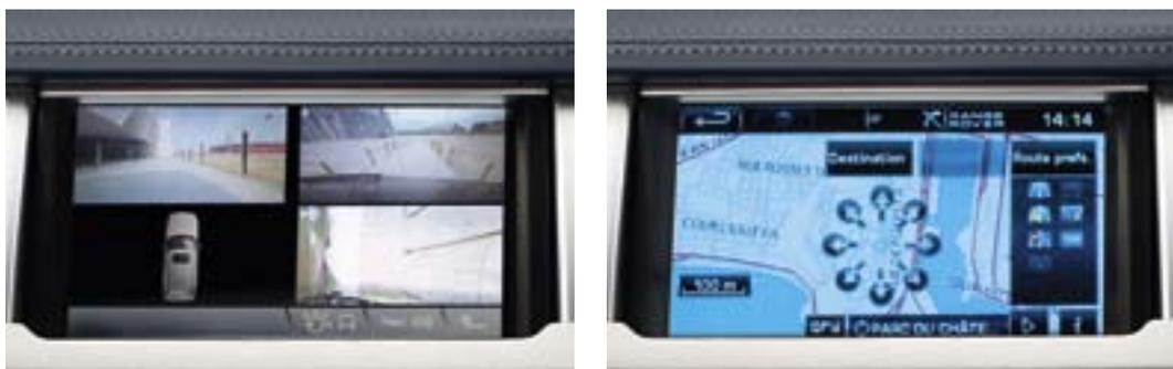
Five digital cameras are housed around the vehicle; two on either side of the front bumper, one in each of the door mirror casings and one in the rear spoiler.
