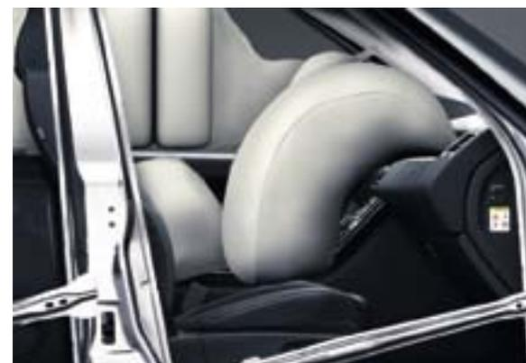
Further improvements to the stability control systems include Roll Stability Control and Enhanced Understeer Control. Range Rover Sport displays real strength in impact tests, thanks to its hydroformed frame design and advanced engineering. For added peace of mind the vehicle is equipped with front and side curtain airbags that are fitted to protect both front and rear passengers.
