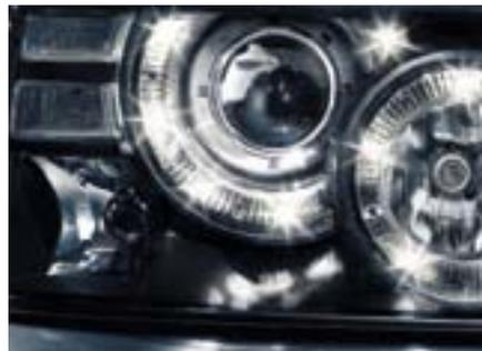
Xenon Headlights with LED technology and Range Rover signature 'concentric circle' design give Range Rover Sport a striking headlight identity. Automatic Headlights with optional High Beam Assist detect vehicle headlights/tail lights and dip the high beam.
