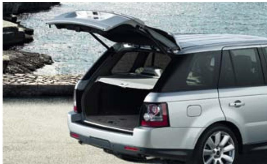
The power tailgate adds practicality and makes life with your Range Rover Sport even easier. Opened at the touch of a button on either the fascia or key fob, the opening height is programmable to suit personal preferences and accommodate more confined loading areas. The tailgate is closed via a button on the inside of the trunk lid.
